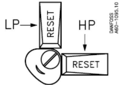
If the lockout is caused by the controls high side cut out, allow the pressure to drop at least 60 PSI below the cut out set point press and release the HP RESET button on the top of the control to restore operation of the chiller.
